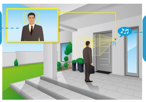
The camera will sound a ring when a person is detected on the front door. And send notification to your smart phone
