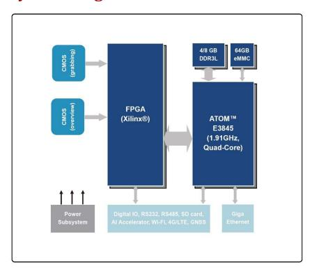
Smart camera is a programmable imaging platform. It integrates image sensor, high-speed CPU, FPGA image pre-processing unit, mass storage and Ethernet interface, etc.
